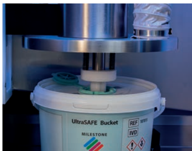
Formalin is added until the preset ratio is achieved (formalin/weight of specimen)
