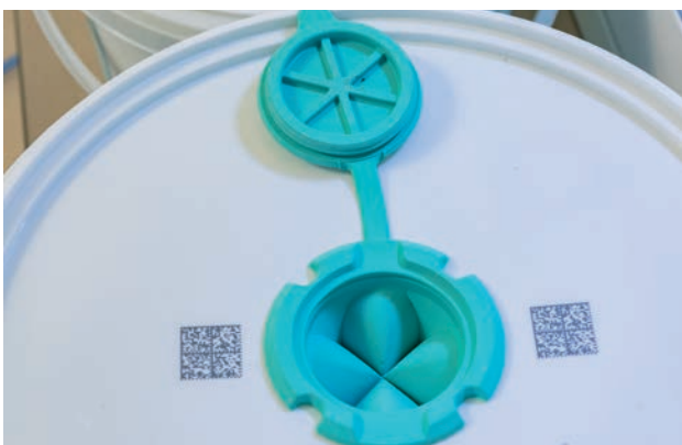
Quadricuspid valve during operation
