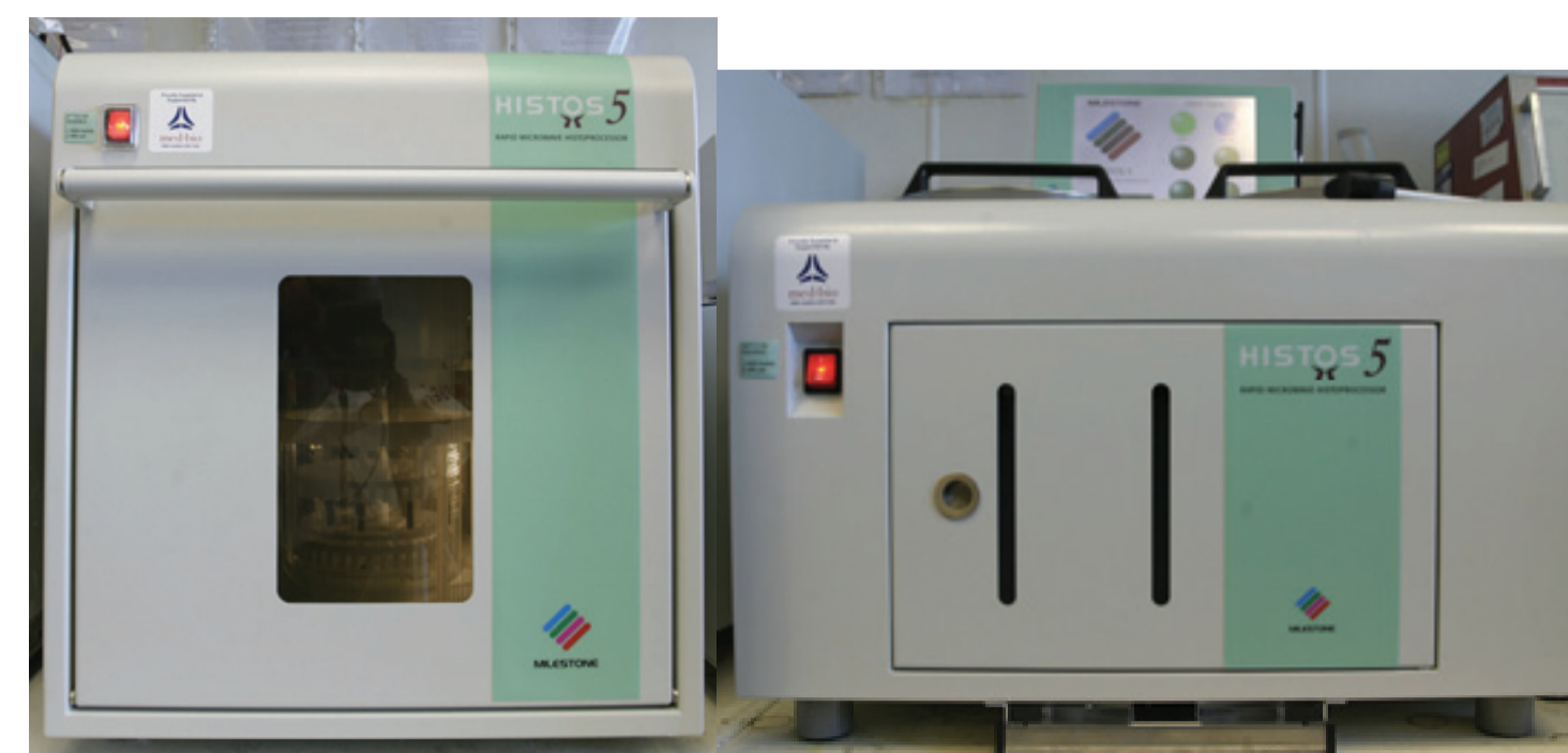
Fig. 1 Milestone Histos 5 Microwave Tissue processor. The Microwave retort is on the left side. The unit on the right has the vacuum retort and the wax retort.
