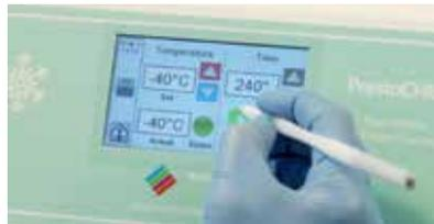
**2** Freeze the specimen at -40°C for 4 minutes.
