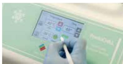
**5** Start a second freezing step for 1 minute. Transfer the specimen to the cryostat.
