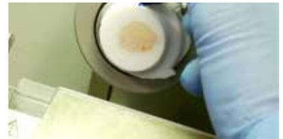
**3** Rapidly transfer the specimen to the cryostat kept at a temperature of -20°C or below. Rapidly trim the specimen.
