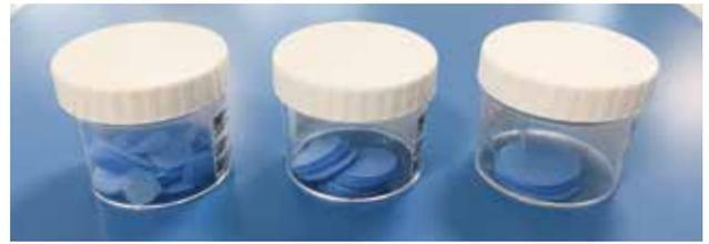
Lens paper disks are an excellent support for freezing small fragments or delicated specimens making the difficult task simple and rapid. Available in 3 sizes (diameters of 16, 22, 30 mm).
