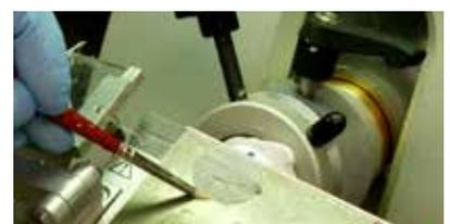
**6** Immediately start cutting with a rapid movement of the wheel.
