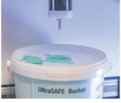
Formalin dispenses based on the preset, selected formalin/specimen weight ratio
