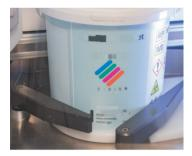
The bucket automatically centers and the built-in scale records the specimen weight
