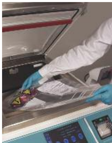
Following genomic sampling, the SealSAFE instrument adds a fixed volume of formalin to the specimen in a bag, which is then resealed and stored.
