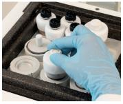
Add the chuck on top of the mold and then add the heat extractor on top of the chuck
