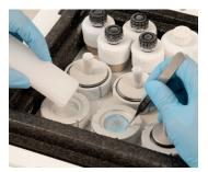
Gently transfer the specimen from the spatula to the bottom of the empty mold
