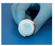
Remove the chuck from the mold. A block with a perfectly flat plane surface is ready for trimming
