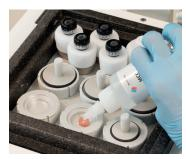
Use Milestone's cryoembedding compound (MCC) and fill the mold to the top
