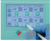
Choose the time depending on specimen type and start the timer (typically 60 seconds)
