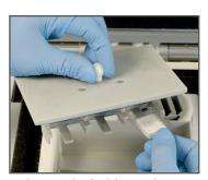
Take out the holder and carefully slide each of the cryomolds from the holder
