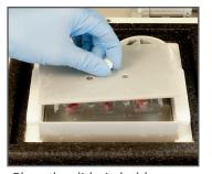
Place the slide-in holder on top of the tank. The fluid inside will freeze the mold
