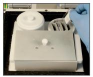
Once removed, you can store up to 6 cryomolds in the holder inside the chamber
