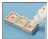
Using Milestone's MCC (cryoembedding compound), fill each cryomold to the top
