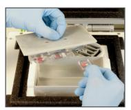
Positon each of the cryomolds into the holder by gently sliding them in
