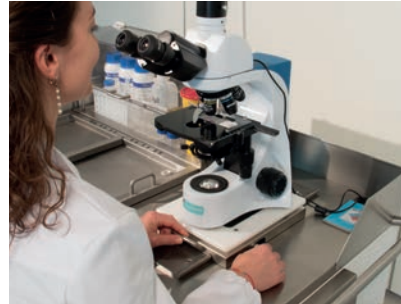
Adjustable microscope sleigh for ergonomic movement forward-backward
